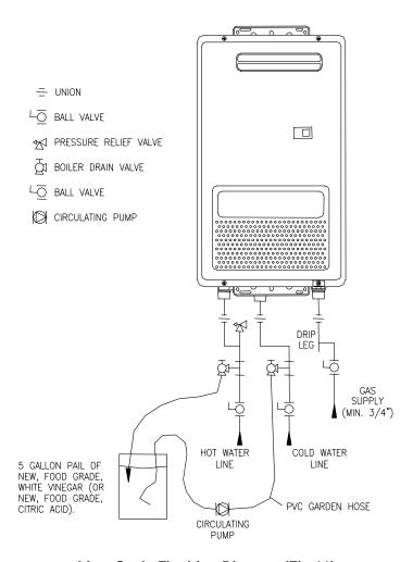
**Lime Scale Flushing Diagram (Fig 11)**
